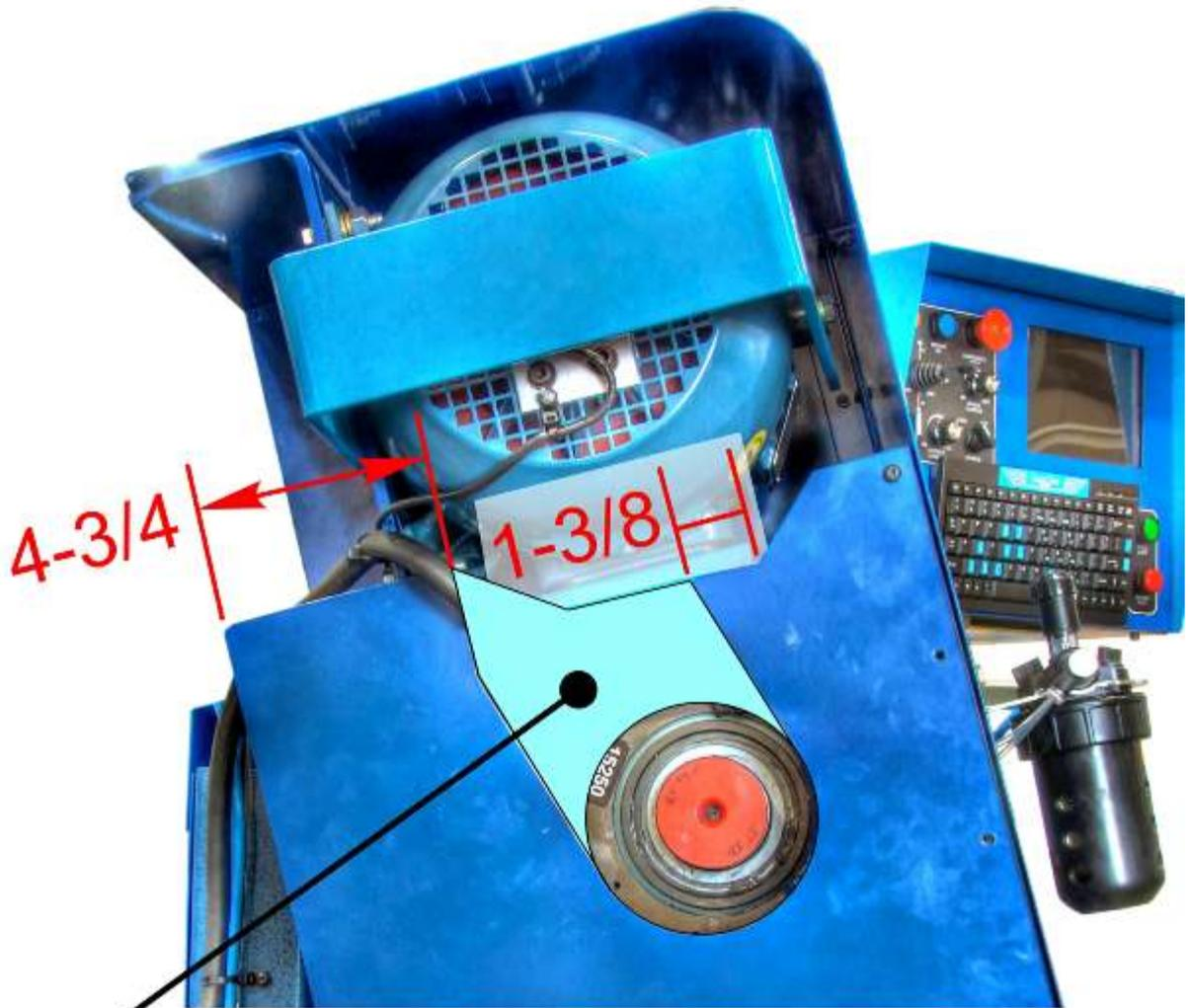
Remove this section to allow the Zip Loader tray to pivot for spindle liner replacement.
