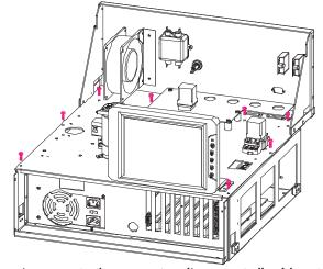
To gain access to the computer, disconnect all cables at rear of CNC, remove eight screws and set chassis asside
