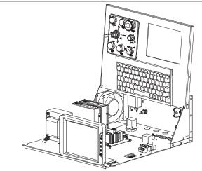
It is not necessary to disconnect cables to front-panel. Stow panel in notches at rear of top chassis as shown.
