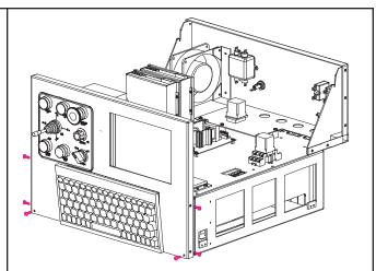
Remove six screws holding front panel.
