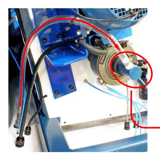
Through-spindle coolant option is very effective for clearing chips while boring, grooving or threading id holes.
