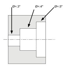
For this example, three diameters have to be turned with only one tool. Each of the diameters can have an individual offset.
