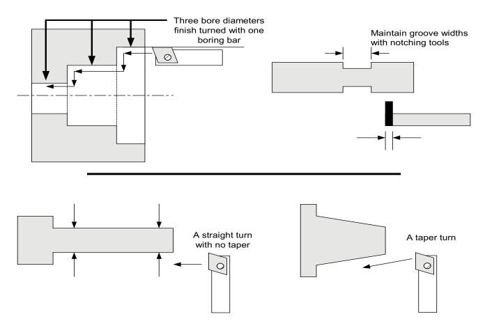
In all three cases it would be very advantageous to be able to have the operator make corrections to the parts that entail more than just moving the tool by changing the tool offset (T). If you made a change to the tool offset, the overall size of the part would change in each of the above examples.
