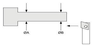
With this shaft, 0A diameter = 0B diameter. In order to do this, put an offset command at the end of the turn.
