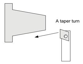
The actual taper that a tool cuts will depend on the toolnose radius. If this is not an easy tool to maintain then the taper will vary as the tool changes. Normally this would be a big problem. However with the secondary offsets this is very simple. We could put a secondary offset at the end of the taper and then turn the offset off. This would look like:
