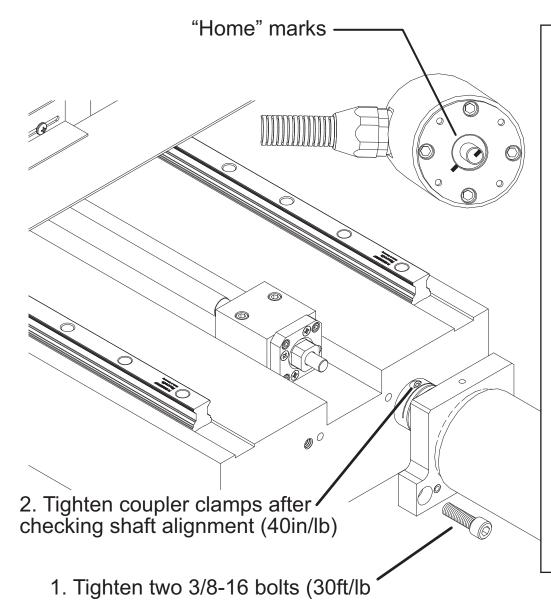
Notice the mark on the end of the motor shaft and another on the face of the motor. These marks are aligned when the motor is at "home". Turn the motor shaft so that the marks are 180° apart; that is 1/2 turn. This provides about 0.100" clearance past home.
